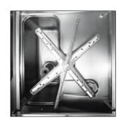
The rotating 4 spoke wash arms create a deflection off the internal walls, and thereby intensify the wash action.
