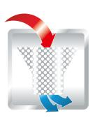
The fine filter system GENIUS-X<sup>2</sup>, with integrated pre-washing process, filters the wash water continuously and then pumps out the soil particles.
